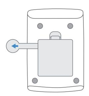
**Remove the plastic tab** from the battery compartment.
